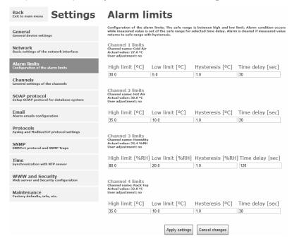
Example of setting the limit to the upper alarm limit:
